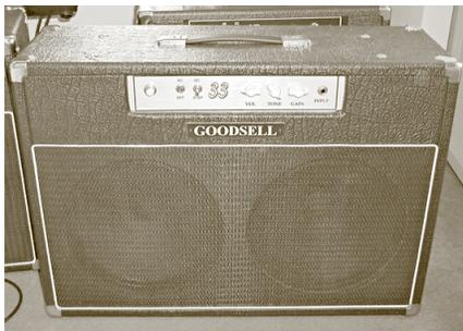
The first significant departure from the 17 was the 33, which was (and still is) basically the same amp with twice the tubes and power. These were
